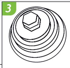
3 Tighten to 10 Newtons, or sufficient tension to prevent filler unscrewing when cap is removed
