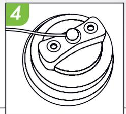
4 Install screw cap, and fasten the tether
